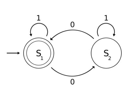
**Moore Machine**. Edge labeled with i=input.  $S_1$  is the start state (arrow from outside) and the accept state (double circle). The language recognized by M is 1\*(0(1\*)0(1\*))\*
