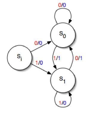
**Mealy Machine**. Edge labeled with i/o, i=input, o=output. Suppose S<sub>i</sub> is the start. **What** is the input/output relation?
